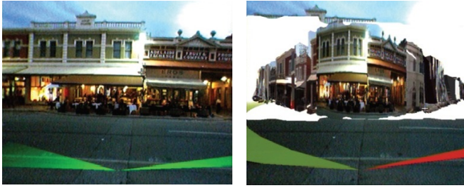
Fig. 15. An original image (left) is distorted (right) to reveal hidden structures located outside of the current view. (Sandor et al. [150] ©[2009] IEEE). The original images were minimally adapted to fit on this figure.
